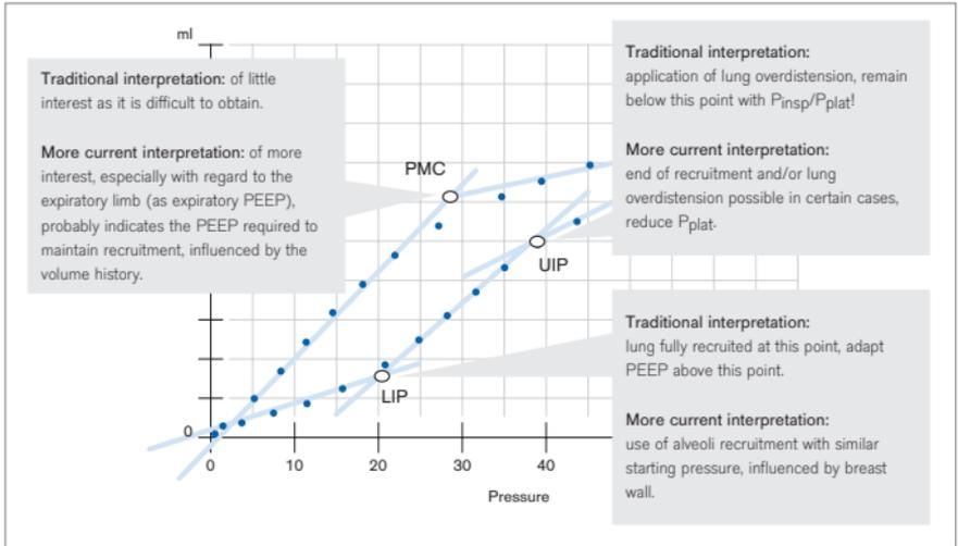
Fig. 1 Information from the Low Flow manoeuvre
