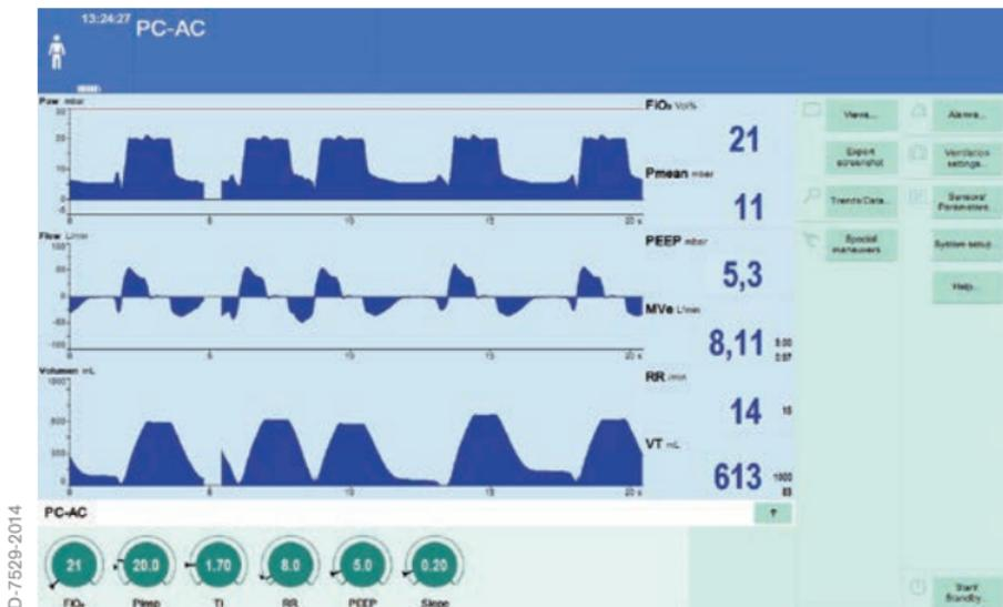
Fig. 2 (PC-AC with triggered and untriggered mechanical breaths)
