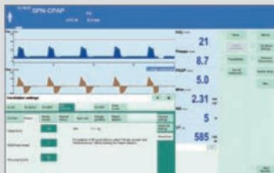
**!** *SmartCare/PS can be started with any PEEP setting between 0 and 20 mbar and with any selected  $FiO_2$  concentration. The spontaneous breathing test starts once the target support pressure ( $\Delta P_{supp}$  target, see 2.) has been reached and the PEEP and  $FiO_2$  values set by the user have been reached or undercut.*
