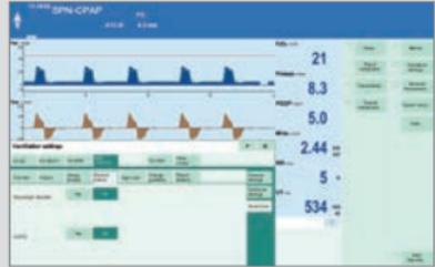
**!** The COPD “Yes” setting means that the SmartCare/PS continues to accept  $\text{etCO}_2$  values less than or equal to 64 mmHg (8.5Kpa) as normal. This may also be helpful for patients with permissive hypercapnia. The neurological disorder “Yes” setting means that the SmartCare/PS continues to accept respiratory rates of up to 34/min as normal. This may also be helpful for patients with higher respiratory drive.
